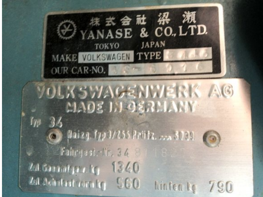
Above: The spare tire area of Japanese T34s featured a special Yanase ID plate fitted above the VW body ID plate.
